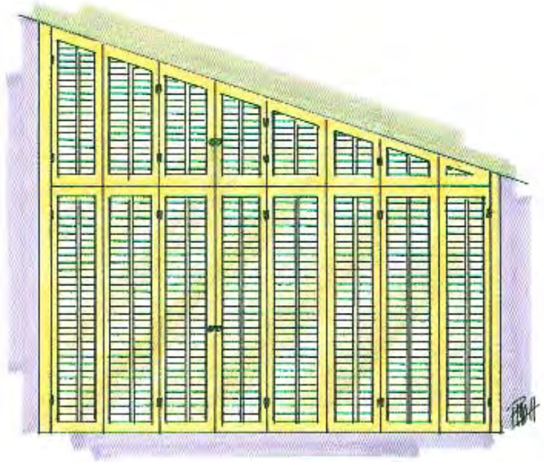
Shutters Custom Fitted to Slanted Clerestory Window
