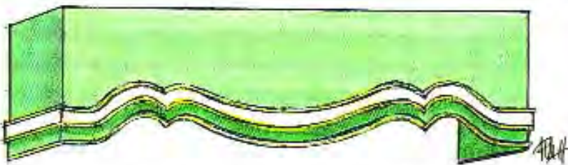
Cornice with Shaped and Raised Banding
