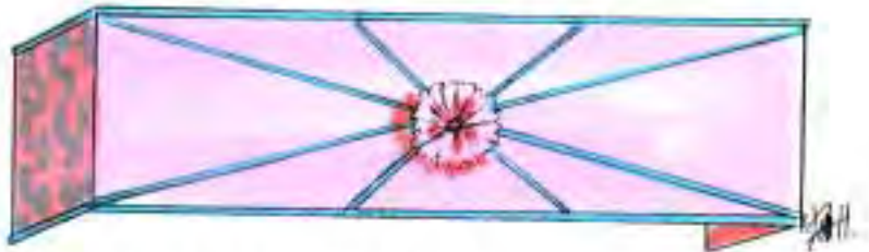
Straight Cornice with Diagonal Welts and Center Rosette
